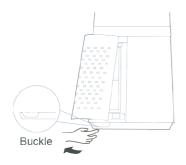
2 Take out the pre-filter Press the raised part on both sides to pull it outwards, and take out the pre-filter.
